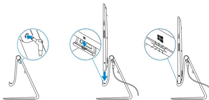
**NOTE:** The docking-status light on the powered stand turns on when your computer is correctly seated.
